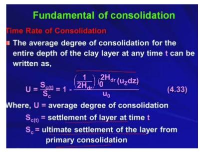
Now the average now basically you have seen that degree of consolidation is varying with depth right. So, degree of consolidation is not a constant for the whole deposit. So, if I consider this is my soil deposit or the clay deposit, saturated clay deposit, I cannot say my degree of consolidation is at a particular time my degree of consolidation is constant for the whole deposit no right. Already we have seen.
