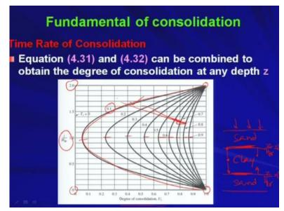
So, equation 4.31 that means the equation what was giving me the excess pore water pressure in terms of say initial excess pore water pressure and say time factor all those things that is the fundamental equation. So, that equation 4.31 and just now whatever we have seen equation 4.32 can be combined to obtain the degree of consolidation at any depth z am I right.
