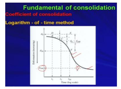
So, now basically if we look at the figure whatever I said you so this is the curve okay so this is your E or the deformation so E nothing but proportional to deformation right. So, deformation versus time scale okay. So, now basically we are plotting that thing with time scale okay, so deformation versus time. Now I mean as deformation increases right your as time increases rather the deformation also increases.
