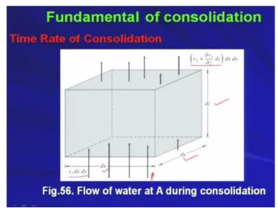
Now we are considering any say soil element okay some 3 dimensional soil element we are considering in the clay deposit so which is having the dimensions dz in the z direction dy in the y direction and dx in the x direction. So, dx, dy, dz is the total volume dx into dy into dz is the total volume of this soil element. Now we are considering 1D flow that means the flow will be only in the one direction as that is another assumption in the 1D consolidation theory establishment right.
