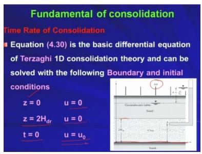
So, equation 4.30 is the basic differential equation of Terzaghi 1D consolidation theory and can be solved with the following boundary and initial conditions. So, what are the different boundary and initial conditions? At z equal to 0 so this is the first boundary condition at z equal to 0 that means you are here okay. What is your excess pore water pressure? That must be 0 because that is the interphase between the clay and sand layer.
