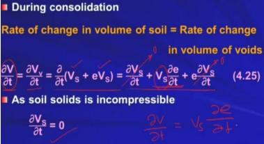
Now during consolidation, rate of change in volume of soil is equal to rate of change in volume of voids. Already several times we have discussed this thing. So, volume of soil whatever change is happening in the volume of soil that is nothing but equal to the volume of I mean change in volume of voids right. So, if that is true so del v dt that is the rate of change in volume of soil is equal to del V v by dt del t.
