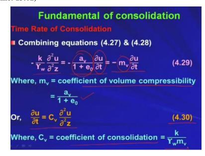
Now combining equations 4.27 and 4.28 now we can get so this was there earlier. Now we can write that is minus a v into 1 plus e not into del you del t. So, if you go back so del e del t in place of that we can write down this del u del t. In place of del e del t we can write down del u del t minus a v into del u del t right. That is nothing but equal to minus m v into del u del t where m v is the coefficient of volume compressibility and is equal to a v by 1 plus e not okay.
