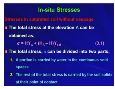
So, the total stress at the elevation A can be obtained as, so the total stress means the whatever stress at elevation A, what is A, if you look at so at this point basically we are trying to find out the total stress. So, the total stress at elevation A can be obtained as sigma that is the total stress is equal to H, H into gamma w. What is H? H is nothing but the depth of water on top of the soil top surface right. So, that is the depth of free water basically okay.
