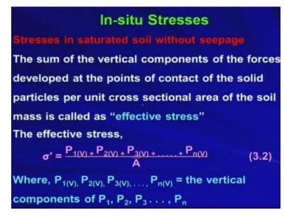
Now the sum of the vertical components of the forces developed at the points of contact of the solid particles per unit cross sectional area of the soil mass is called as effective stress. So, that means the effective stress is purely the property of the soil grain. Now the soil grain basically soil particles they are transferring the stresses through its contact point okay and these stresses will be known as the effective stress.
