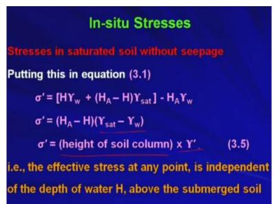
Now putting this in equation 3.1 so sigma is equal to sigma prime plus u. If you put that thing in equation 1 so basically you will be getting sigma prime in this fashion. So, sigma prime is equal to H into gamma w plus H A minus H into gamma saturated minus H A into gamma w so from that you can get sigma prime equal to H A minus H into gamma sat minus gamma w. Now what is H A - H so that is nothing but height of soil column right.
