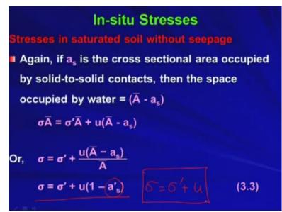
Now again if small a s is the cross-sectional area occupied by solid-to-solid contacts then the space occupied by water is total cross-sectional area is A bar minus the solid-to-solid contact area is say small s so A bar minus a s is nothing but the area or the space occupied by the water as simple as that.
