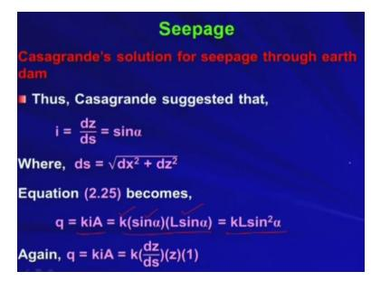
So, the modification is suggested by Casagrande and he suggested that i should be equal to dz ds okay. So, now instead of taking dz dx you are taking dz ds. What is s? s is nothing but the surface or the parabolic or the Phreatic line surface okay. So, that ds dz by ds is nothing but equal to sin alpha if you go back to the previous figure you will see that dz by ds is nothing but sin alpha.
