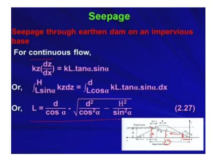
So, now this for continuous flow I mean if you want to satisfy the equation of continuity and for the continuous flow whatever flow is happening through this section bf the same amount of flow will be happening in the section through the section ce, there is no issues because whatever flow is entering the section bf the same amount of flow or same amount of seepage will be going out from through section ce.
