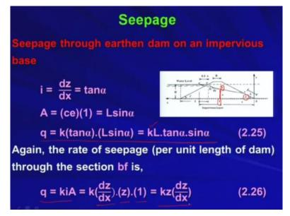
That is rate of seepage is given by k into L into tan alpha sin alpha where alpha is nothing but the slope of the downstream phase that is given by this figure and k is the coefficient of permeability whereas L is completely unknown to me as I told you in the last lecture that L is not known to me so I need to find out L. Now again so the rate of seepage per unit length of dam through the section bf any section say any section in between say that is bf okay.
