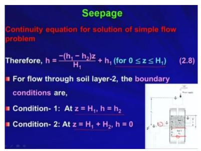
So, for that I need the boundary conditions right to obtain A 1 and A 2. For flow through the soil layer 1 the boundary conditions are, first condition is at z equal to 0, if you recall the figure at z
