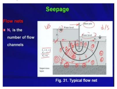
Now let us see so now we will see some typical flow net. This is another barrier what is nothing but sheet pile so it will not allow the flow from upstream to downstream like this, but however the flow can occur below the soil deposit okay. So now this is the water level on the upstream side, this is the water level on the downstream side. So now ab is basically the bed level on the upstream side whereas d is the bed level on the downstream side.
