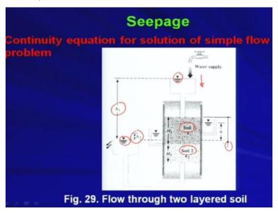
So, in this problem basically you have 2 different soil layer, soil 1 and soil 2. Soil 1 is having the height of the sample say capital H and whereas soil 2 is having the height H 2; k 1 and k 2 are the hydraulic conductivity of soil 1 and soil 2 respectively. So basically, what we are doing, we are putting water okay and basically that is at the entry level this is the head can be measured from this and at the exit level the head is measured here.
