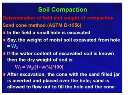
Now in the field where you have compacted the soil and where actually you need to find out the unit weight, so basically in the field you excavate a small hole okay that is I mean comparatively reasonably small hole you just excavate okay and say the weight of moist soil excavated from hole is W2. So, whatever soil you have excavated from the hole, say the weight of that moist soil is W2 because you have compacted so the soil will be moist.
