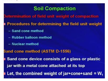
First one was the sand cone method, then rubber balloon method, and nuclear method. So, among these 3 we will be talking about the sand cone method which is as per (ASTM D-1556). So, basically in the sand cone device consists of a glass or plastic jar with a metal cone attached at tips right. So, you will be having one jar which will be made of glass or plastic and on top of that you will be having some metal cone.
