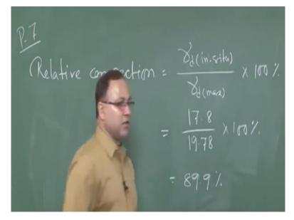
So, we can write down the relative compaction. What will be the expression for relative compaction? From the definition, itself we can you can see that that whatever you have achieved and whatever was there, based on that you can calculate the relative compaction. So, that is nothing but gamma d in-situ by gamma d max, or by if you want to express that thing in percentage multiply by 100.
