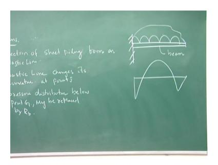
What are the assumptions the basic assumptions deflection of the seat playing hallmark elastic line deflection of a sheet piling form an elastic line then elastic line changes its curvature elastic line changes its curvature at point j. So, this area the course below g pressure distribution below point g may be replaced by r b may be replaced by reaction force r b
