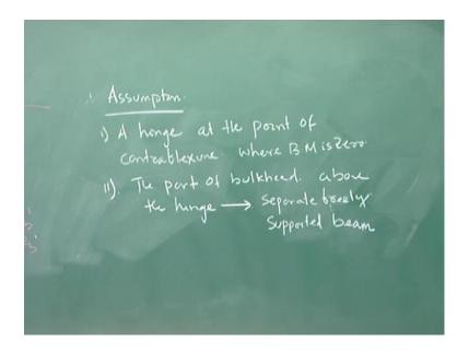
If I summarize it what are the assumption a hinge at the point of point of contra flexure at the point of contra flexure where bending moment is zero. Then the pat of bulk head above the hinge can be treated as separate freely supported beam can be treated as can be treated as separate freely supported beam or you can say that can be treated as freely supported overall beam or freely supported beam. We have some r b dash acting at the hinge can be evaluated and these r b what is the procedure.
