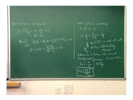
Which is equal to passive minus active at point d which is equal to two c minus q minus two c which is equal to four c minus q. Now you got how this four c minus q term has come. Now we can get it, this has been derived, this is your passive earth pressure minus active earth pressure. This is coming four c minus q let us consider the result and of this
