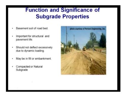
So, basically we start with this function, and significance of subgrade properties that will it is come under basement of soil of road bed, and important for structural, and pavement life should not deflect excessively due to dynamic loading may be in fill or embackment compacted or natural subgrade.
