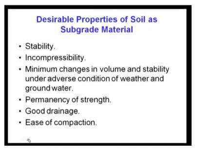
Now, desirable properties of soil as subgrade material its based on stability incompressability minimum changes in volume, and stability under adverse condition of weather, and groumd water, then permanency of strength good drainege, then eazy or ease compaction.
