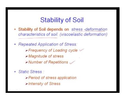
Stability of soil, if you look at the styability of soil it depends upon stress deformation characteristics of soil stability of soil is depends on the stress deformation characteristics of soilthat means viscoelastic deformation viscoelastic deformationrepeated application of stress repeated; that means, repeated note generally applied by means of trafic loading repeated load means suppose there are n number of vichcle passes in the road; that
