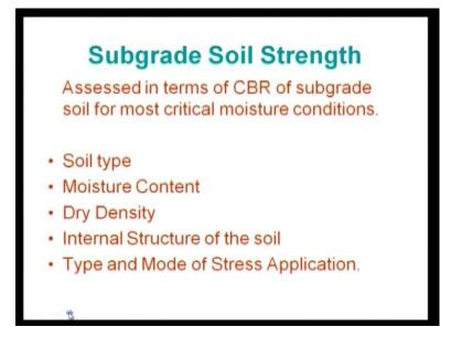
Then subgrade soil strength that is assessed in terms of c b r of subgrades soil for most critical moisture conditions strength has to be measured by by means of c b r califormia bearing ratio test this strength has to be measured; that means, soiled type moisture content dry density internal structure of the soil type, and mode of stress application.
