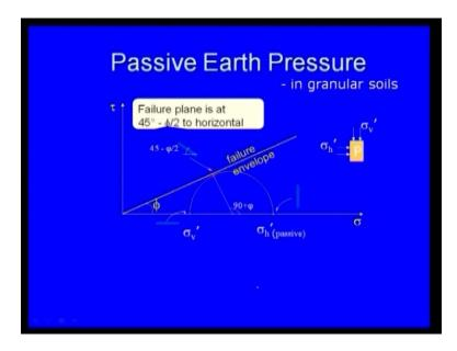
Now passive earth pressure in granular soil, so failure plane is at 45 degree minus phi by 2 to the horizontal. So this is your sigma v prime, this is your sigma v prime, sigma v prime and sigma h prime passive state.
