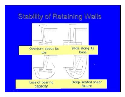
Then different failure of your retaining wall or stability analysis of retaining wall, we have already also discussed. Overturning about toe, sliding along its base; this is the overturning above the toe, sliding along the base, loss of bearing capacity, deep-seated shear failure.
