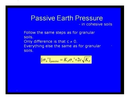
For cohesive soil, these steps are same. For cohesive soil, for calculation of your passive earth pressure, these steps are same like your granular soil. Only difference is that c is not equal to 0, c is not equal to 0, that means cohesion force is not equal to 0 - c is not equal to 0. So sigma h prime passive is equal to K p into sigma v prime plus 2 c root over of K p.
