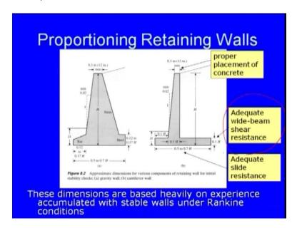
Now proportioning these retaining walls also I have discussed earlier. So proper placement of concrete at the top and adequate width-beam shear resistance, adequate width beam shear resistances then adequate slide resistances.
