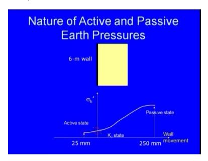
So nature of active and passive earth pressures, suppose you consider a 6 meter of wall, so this is your value of K 0 state at rest, so you can say that active state it comes about to be 25 mm then passive state, it comes about to be 250 mm. How this nature of active and passive earth pressure is varying from active to passive state. This is the variation.
