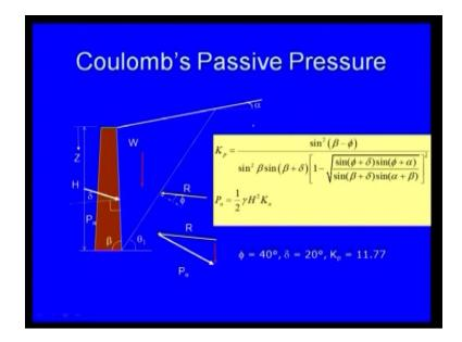
Now Coulomb's passive ah pressure, the K p this things I said earlier also ah P a is equal to half gamma H square into K a. Suppose, for example, if you take the value of phi is equal to 40 degree, suppose this is a back field soil of inter frictional angle of this soil, phi is equal to 40 degree, delta that means coefficient of friction between soil and wall is equal to 20 degree, so K p value comes out to be 11.77.
