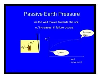
Passive earth pressure now if you would take at this as the wall moves towards the soil, that means sigma h, sigma h is increases. This wall is moving towards that means wall is generating pressure towards this field till the failure that means this is your K zero condition that means
