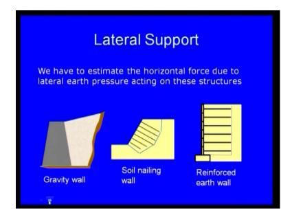
Now, lateral support this retaining wall, if you look at there is a gravity wall soil nailing
