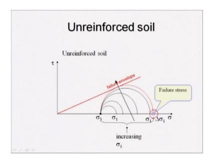
Now, for unreinforced soil this is my failure envelop now the movement we increase increasing; that means, if you look at this increasing in sigma one this failure stress be this more circle we increasing to will failure envelop this is your failure stress sigma one pulse delta sigma one.
