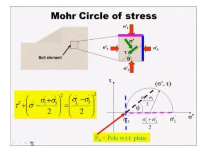
Up to last class. So, we are finish this basic about your a, and stresses in the solve must now continues with this more, and circle stresses. We have discourse this what is the pole with respect to pole. We can find it out the failure envelope, and this sigma in tu at failure.
