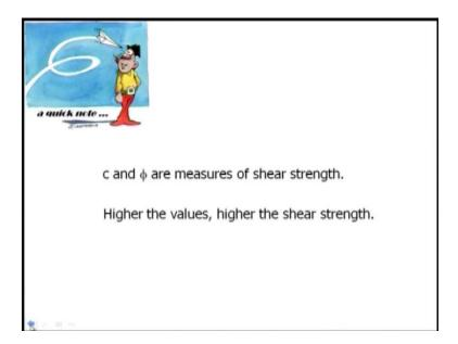
A quick note c and phi are measures of shear strength. Higher the value means higher the value of c and phi, higher the shear strength, higher is your shear strength.
