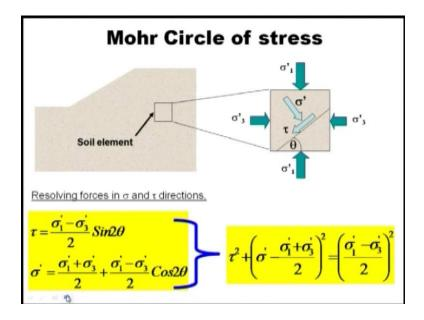
Mohr circle of stress. If this is your soil element, if you take it soil element in the soil mass, then this will your sigma one prime and sigma three prime. And with this, a theta then you are getting tau and sigma prime. Resolving forces in sigma and tau directions, you will get it tau is equal to
