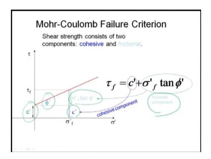
So Mohr-Coulomb failure criterion, shear strength consists of two components; cohesive and frictional. This part is your intercept cohesion, and angle is your friction. So tau f is equal to c prime, c prime sigma prime f tan phi prime. So as I said c prime is your cohesion component, and sigma f tan phi prime is your, this part is your sigma phi tan phi, this is your sigma prime tan phi prime. This is your frictional component and this part is your c prime, this is your cohesion component.
