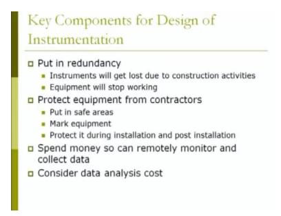
Then key components for design of instrumentation that means put in redundancy that means instrumentation will get lost due to construction activities and equipment will stop working. So protect equipment from the contractors that means put in safe areas, mark equipment, and protect it during installation and post installation. Then last is your spend money so can remotely monitor and collect data. And consider data analysis cost also. This part also you have to taken into consider.
