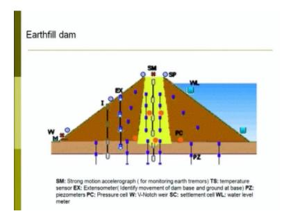
Then similar kind of also, there is another also earth fill dam, one is your, this is your rock fill dam, second is your earth fill dam. In this case of earth fill dam, in the core if this is the core, this is your core part, in this core, you have yoru SM – strong motion accelerograph. And you have also your SP and as well as your ah pressure meters. All virtual instrument has been placed ah in case of earth fill dam in the core.
