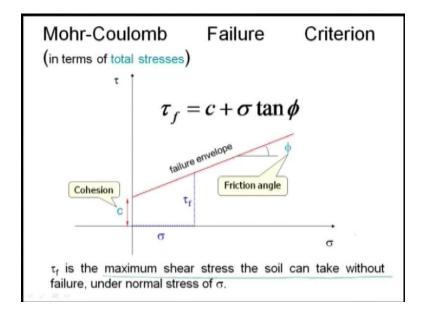
Mohr-Coulomb failure criterion that means in terms of total stresses if I draw the Mohr-Coulomb failure criteria that means tau f is equal to c plus sigma tan phi. C is your cohesion and tau f is your failure envelope and phi is your frictional angle. Tau f is your maximum shear stress the soil can take without failure, tau is your maximum shear stress, soil can take without failure, under normal stress of sigma.
