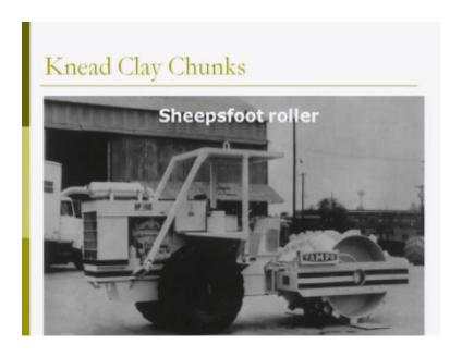
Look at this how this it foot a sheep foot sheep foot roller it looks like, if you look at this it put rollers there are there are just threaded parts around the periphery of the roller. So, that it has been used particularly for clay soil, because it has a high cohesive.
