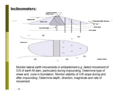
Second part is your second part is your inclinometer, if you look at the inclinometer inclinometer what happened it measure your where there this sloop a stable is there in lateral
