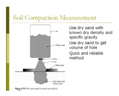
Now, in this in case of a soil compaction measurement by means of sand core method a used dry sand with known dry density. If you using by means of sand replacement method in this case what you are going to do use a dry sand use dry sand with known dry density before you are using this method you should known what is the dry density of that sand, and
