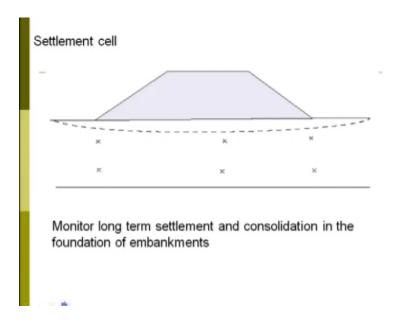
As I said monitor long term settlement, and consolidation in the foundation embankment this is an embankment foundation embankment it place the settlement sail. So, it can measure long term a particularly long term settlement.
