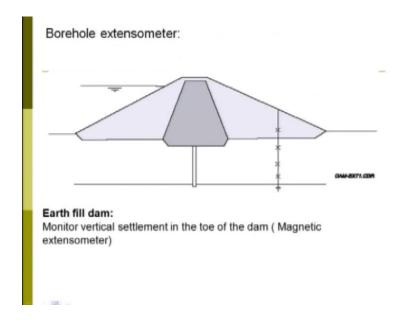
A generally it has been used in, if you look at here this is called bore hole extensometer monitor verticals settlement particularly earth fill dam in the toe the dam in the toe the dam, if this the hill this is the toe in the toe of the dam, it can measure your vertical settlement monitor settlement to determine where there construction can continue or not.
