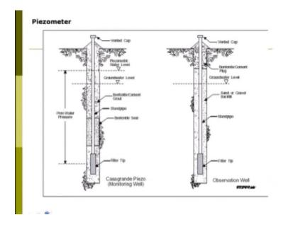
Monitors piezometers a piezometers generally if you look at this piezometer how it looks particularly piezometer its a it is a constructional view, and piezometer water pressure has been given a there is a stand pipe, then ventonites cement grout has been done, then there is a filter tip, then a it has been connected with the vented cap means detail view of your piezometers has been a it has been zone.
