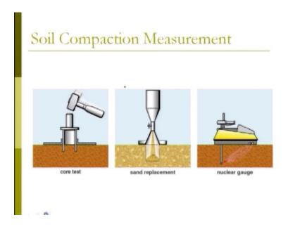
Now, soil compaction measurement how do you measure its soil compaction measurement there are different web different a, as I said earlier one is your core test of there is your sand replacement method, and third is your nuclear gauge this is your nuclear gauge method.
