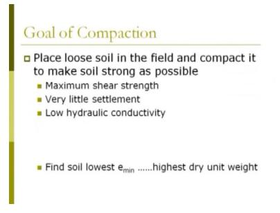
And place a loose soil in the field, and compact it to makes soil strong as for as possible. So, that you will get maximum shear strength, and very little settlement, and low hydraulic conductivity or soil lowest aim highest dry unit weight.
