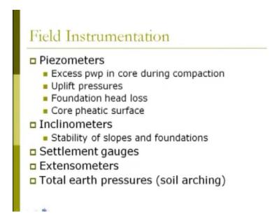
Field instrumentations: There are different field instrumentation; one is your piezometers, piezometer generally use to measure excess for water pressure p w p; p w p is your core
