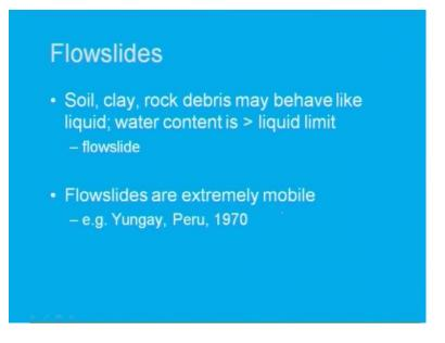
Then flow slides soil clay rock debris may behave like liquid it may behave like liquid water content. So, means behave like liquid, if water content is greater than liquid limit,
