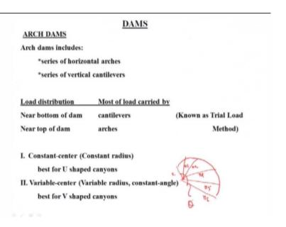
Particularly arch dams it includes series of horizontal arches, and series of vertical cantilevers load distribution most load distribution near bottom of dam near top of the dam, and most load carried by cantilevers arches known as trial load method. So, constant center; that means, constant radius. If I look at the types of the earth one is constant center; that means, this is a constant center this radius is the radius is constant.
