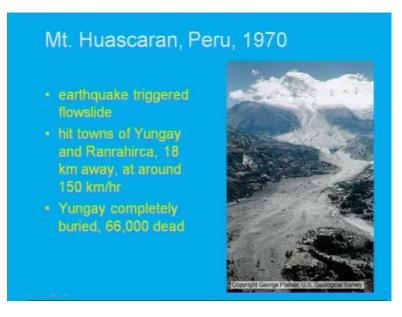
If you look at here peru nineteen seventy earthquake triggers particularly flow slides means what will happen the water, because of earthquake triggered this water content increase this water content is more than water content is more than your liquid limit. So, once is water content is more than liquid limit, if these by means of in peru nineteen seventy by triggering.
