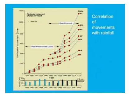
There is there is a like correlation of movement with this rain fall they have given. So, that is out of contains those I am showing with the rainfall how much the movement can be possible, let has been some correlation has been given.
