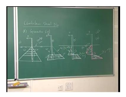
Now we are doing the derivation for cantilever sheet pile. First case is your for granular soil. Now as I say there will be a point of rotation in case of granular soil for cantilever sheet piles, if this is my point of rotation 'o'. The next stage how this derivation has been derived if I so this is acted upon by horizontal load H, k p minus k a line. This is your horizontal force.
