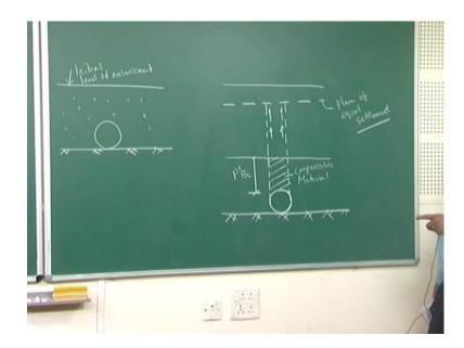
So, if I starts with the a one if I draw the figure a, and b how it looks. So, this is your initial level of embankment, you can say that initial level of embankment, then second one is if you look at here second one is this is your top of final emb embankment and this part is your as I said plane of equal settlement, and this is where it lies this. If I draw the diagramically the two cases this is your compressivable material.
