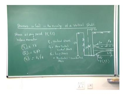
So, what is the stress around the pheripheri of this vertical soft. Let us draw this diagram, this is r zero, and this depth is your a vertical shaft of gamma z gamma z. Now stresses in
