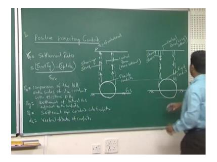
Let me to rigid a ratio called settlement ratio this is called r p r p this is not gamma this is a r p called settlement ratio which is equal to delta m plus delta g minus delta f plus d c by delta m. So, delta m is your let me defined it delta m is equal to compression of the fill compression of the fill on the sides of the conduits in the distance p b c.
