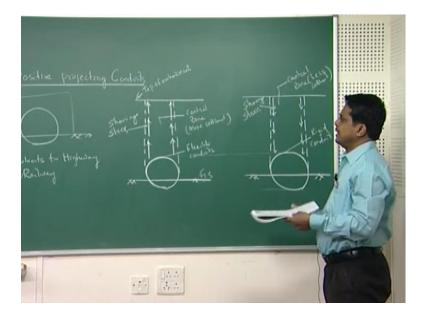
Let us start with the second one this is your positive projecting conduits projecting conduits means it will be race, it will look at here it will race. For example, why it is called positive projecting conduit, if you look at here exhaust light embedded bellow the ground surface, and it will this pipe or the conduit, it will above of the ground circle above of the ground circle that is why it is projecting this some part is projecting above of the surface.
