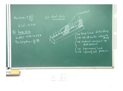
Now, maximum Pending movement, now maximum Pending movement which is equal to plus minus pl square by twelve, because this is a continuous slab with the supports are there. So, it will p l square by twelve, and based on this maximum bending movement as I have discussed once you get maximum bending movement these has to be equated to q b d square is equal to maximum
