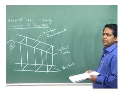
Now, vertical ties connecting counter fort, and heel slab you see why I am discussing these these counter forts these counter forts of reinforcement bars has to be connected with your upright slab as well as your heel slabs it has to be connected. So, that it should not be separated after this design is over.
