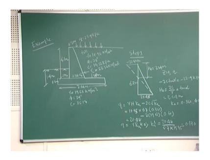
Let us solve one example per kindly bar retaining wall, and its stability analysis check this is the wall, and this dimensions has been given later on we will see where there was no dimensions of wall has been given you will have to start with scratch level.
