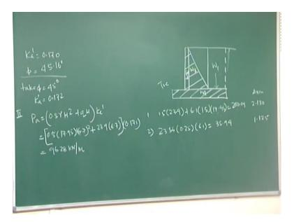
Now, with help of k a prime one seven zero with the modified value of soil we are taking c pile soil to equivalent pile soil with this k a prime coming about zero point one seven zero pie is coming about zero point a forty five point one six degree. Let us take five is
