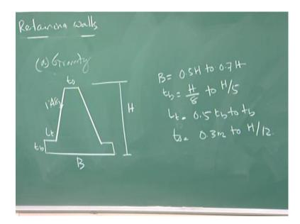
So, base easy equal to gravity retaining wall zero point five base to zero point seven h, and the easy equal to h by eight to h by five t easy equal to zero point five t b to t b, and t zero easy equal to zero point two meter to h by twelve, and minimum back it should one is to forty eight this angle these are all certainty dimension I want give it that. So, you can while starting this kind of this starting this analysis, and stability.
