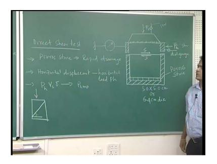
Next part of your, that is direct shear test (( no audio 00:27 to 00:45)). Diagram for direct shear test, I am just drawing (( no audio 00:50 to 05:28)). Next test is your direct shear test. So, direct shear test is (()) size is either 5 by 5 centimeter by 5 centimeter or 6.4 centimeter dia. It may be a circular shape or it may be a square section. If you will look at, this direct shear test cross sectional view. So, this is a shear box.
