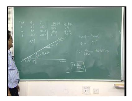
So, there is a given triaxial data. So, this is my test, 1, 2 and 3. Then, sigma three, sigma one is given, this is 40, 80, 120. Then, 103.0, 166.0, then 222.0. Sigma three and sigma one is given. From there, you can find it out, p and q in K p a. So, this will be 71.5, p and q how you will get it, p and q as I said earlier. So, p is equal to sigma one plus sigma
