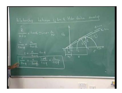
Now, we will go for next part is your relationship between K f line and mohr's failure envelop (( no audio 25:10 to 25:55)). The tangent which touches your mohr circle, that is your, you can say, that is phi line or failure line from you are getting, from your standard triaxial test for three sets of confining pressure. Sigma means sigma three one, sigma three two, sigma three four or three three, but here p q with this stress path, it is passing
