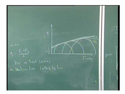
Now, there are, as there are two parameters. So, you have to do minimum two tests to get your result. That means, in that case, shear stress versus normal stress, if I plot it. If I draw the mohr circle, so draw the mohr circle and find it out the common tangent. With this point, draw a tangent, where it touches the mohr circle or the failure point. So, this will give c, and this will give your phi.
