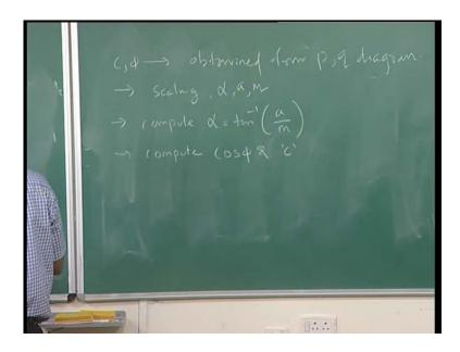
So, c and phi can be obtained from p q diagram. So, that mean this steps, so scaling alpha, a and m. Then, compute alpha is equal to tan inverse a by m. Then compute, cos phi and c. We will do this with a solved example write now.
