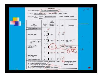
That means what is the scope of the investigation as I said the scope of the investigation you can say that the scope of the investigation is design of two story apartment building, means what purpose you are doing this, so this for design of two story apartment building, this is our scope for that design these are the soil profile calculation has been done
