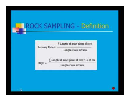
Now, recovery ratio rock sampling length of intact pieces of core divided by length of core advance, length of intact pieces of core, if you look at here length of intact pieces of the core, this is your length of the intact pieces of this core divided by length of core in advance means how much length we are advancing. So, length of intact pieces in core should be greater than equal to 10.16 centimeter, and length of core advance from there you can find it out, what is your recovery ratio?
