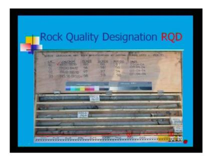
Rock quality designation, that means if you look at this it is IS means 1529 geological and rock investigation, so there are some example coring 1991, 92, 93; length is varying from 188.90, this is 188.90 to 195.05. And rock this ratio recovery ratio you can find it out recovery ratio is your 97 percent, 98 percent, 94 percent, and 98 percent; these are
