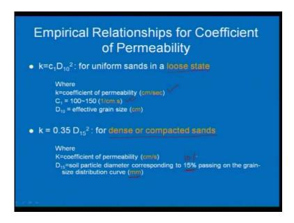
Now, empirical relationship for coefficient of permeability, how to find it out empirically, if you know D 10, D 10 is it is your size of the this means, 10 percent of the particle size finer than that particle, D 10 you can get from your sieve analysis. So, coefficient of permeability k is equal to C 1 into D 10 whole square for uniform sand in loose state; remember, it is in loose state, and this for we are discussing right now for sand.
