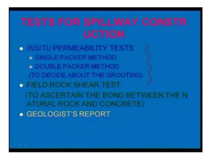
then after construction is over, after few years you can do also post construction, so test for spillway constructions like, you can for irrigation projects you can do because, this is a continues flow of water particularly in irrigation projects. In the soil insitu permeability test you can you will have to determine, because it is related to permeability that is what I am discussing by means of single packer method or double packer method to decide about this grouting.
