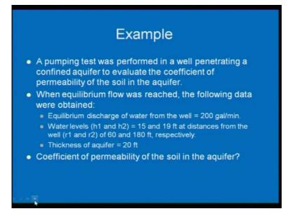
This is a typical example, a pumping test was performed in a well, penetrating a confined aquifer to evaluate the coefficient of permeability of this soil in aquifer; means this has been given data, from there you can find it out coefficient of permeability. So, it is said equilibrium discharge of water from the well is 200 gallon per minute, discharge is generally gallon per minute or c c per minute or c c per second c c per hour.
