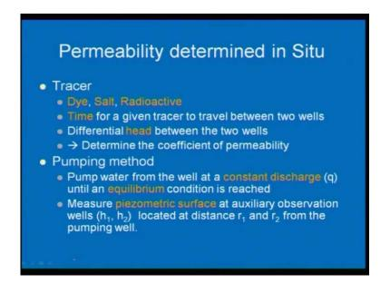
So, tracer is dye or salt or may be a radioactive material, so this can be put inside the soil, inside this water; so that this flow inside the water by means of tracer. You can trace and you can find it out, by means of differential of head between the two wells, you can find it out what is the coefficient of permeability.
