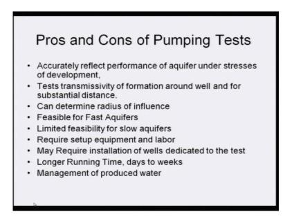
So, I discussed this pumping test, and slug test that means it is say, instantaneous insert of slug into observation wells, either it is a falling head test. Manual and electronic water level measurement before during and after slug insertion, and continued until water level has recovered; and now you come just go back to how this installation of monitoring wells, if you look at here this is a broad picture of how this wells have been installed.
