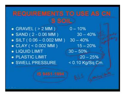
Now, requirement to use as CNS soil, what are the different requirement means, CNS material, if I say CNS cohesive non-swelling soil, if I say how this profile is varying, what kind of material we can say cohesive non non-swelling soil, for this the gradation curve it says gravel should be 0 to 10 percent. How do you decide gravel, in 2 mm, sieve percentage of soil particle retain is about 0 to 10 percent, then we can say that that gravel is about 0 to 10 percent.
