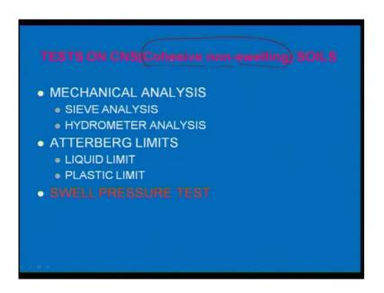
So, mechanical analysis, now it is called test on CNS material or CNS soil, what is CNS? CNS is Cohesive Non-Swelling remember, CNS is nothing but, cohesive non-swelling soil, C for cohesive, N for non, S for swelling, that means we will do test cohesive non-swelling soils generally, it has been used for irrigation projects. So, mechanical analysis we do sieve analysis, and hydrometer analysis, atterberg limits and liquid limits and plastic limits, it has been discussed and swell pressure test.
