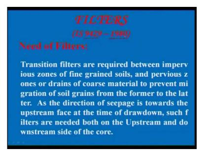
Now, what is as per IS standard, Bureau of Indian Standard, 9429 this is the number, and this is the year 1980, need for filters look at this paragraph. Transition filters are required, between impervious zone of fine grained soil, and pervious zones or drained of coarse material to prevent migration of soil grains from the former to later. As the direction of the seepage is towards the upstream face, at the time of drawdown, such filters are needed both on the upstream and downstream side.
