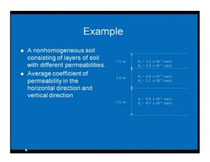
Now, one of the examples, another example a non-homogeneous soil consisting of layers of soil with different permeability, average coefficient of permeability in horizontal, and vertical direction, it has been asked to find it out. So, each layer by means of laboratory test k x and k y you got it, it is 10 to the power minus 3 and 10 to the power minus 4 cm
