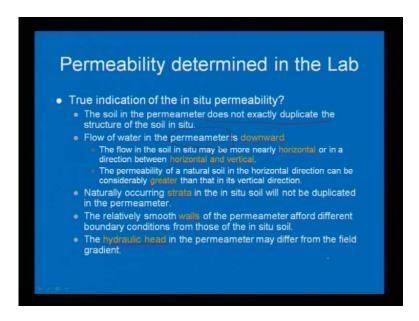
The test equipment by which the test has been conducted this is called permeameter, as I said earlier this is called permeameters. The test equipment where we are going to do this in the lab permeability test this is called permeameter.
