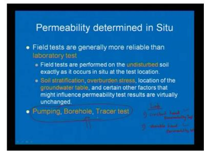
Now, these are the two tests generally we do in the laboratory. What are the test we generally do in the field? The test we generally do in the field, pumping test that means you take pump, certain amount of water leave it and allow water to flow through inside the borehole then measure how much time it takes to flow certain amount of water this is called pumping.
