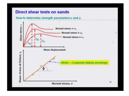
This is your failure, shear stress at failure you will find it out from the peak tau f 3.
