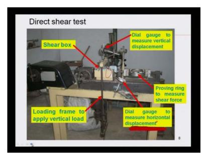
How it has been conducted in the laboratory, just to show this once just slightly repeat of this. This is your shear box, then loading frame to apply vertical load, then dial gauge measure vertical displacement and dial gauge to measure horizontal displacement. And this is your proving ring to measure shear force applied from here.
