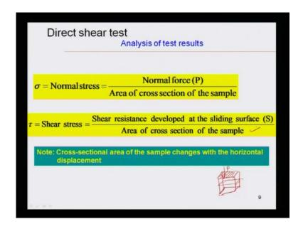
Now, as I said normal stress generally measured normal force by area of cross section, normal stress has been applied by vertically. So, this is the load or normal force p with this area if the direct shear box is like this, this area, this is the area normal force per area that is your normal stress.
