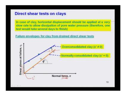
Direct shear test on clay. Now, we have discussed direct shear test on sand. Now, we are going to discuss direct shear test on clays. In case of clay, horizontal displacement should be applied at a very slow rate. If you remember well the displacement laterally horizontal displacement applied to generate your shear stress along the pre defined failure plane.
