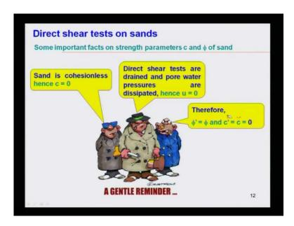
Some important facts on shear strength parameter of c phi of sand, whatever you are getting from direct shear test on sand. Remember sand is a cohesion less soil hence c parameter is to be 0, c is equal to 0. Second case is your direct shear test are drained and pore water pressures are dissipated means as I said earlier direct shear test is almost it gives best result for drained test that means in this case pore water pressure u is equal to 0.
