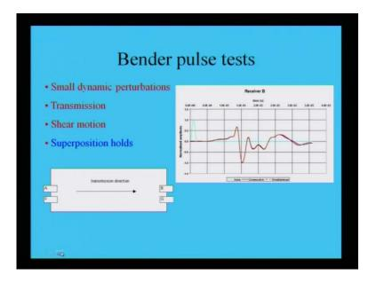
Shear motion and superposition hold if you look at the bender pulse test from transmission direction from source to receiver normalize amplitude in the receiver. If I plot it travel, travel, travel it receive and it go.So, this is a bender pulse test means how this pulse moves inside this soil sample.
