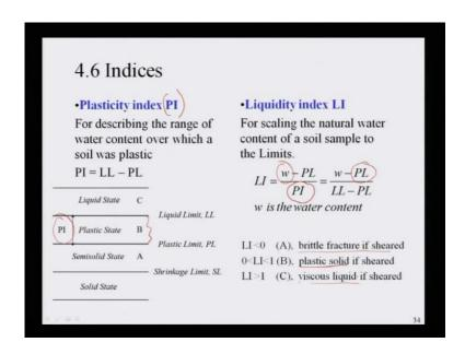
Then we will start this with this liquid limit plastic limit and shrinkage limit. What are the with this limit? What are the parameters we are suppose to get or indices? First one is your plasticity index that is called P I, if it is name P I then it means plasticity index it is describing the range of water content over which the soil is plastic. Once it is said plastic
