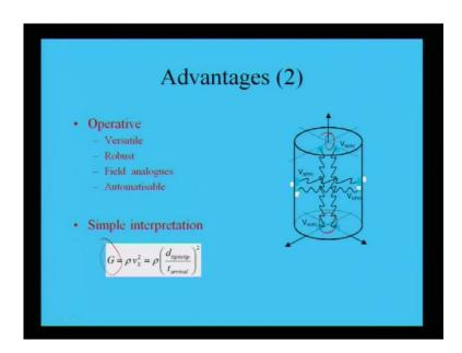
Advantage two is your its operative its means its very versatile and robust and it analogous to your field condition and simple interpretation you can simply interpret. If you look at here my this is my soil that means shear wave has been means if wave has been generated at the bottom by source you receive at the top, that means you can find it out simple interpretation G or shear modulus you can find it out by means of rho in to V s, V s is your shear wave velocity.
