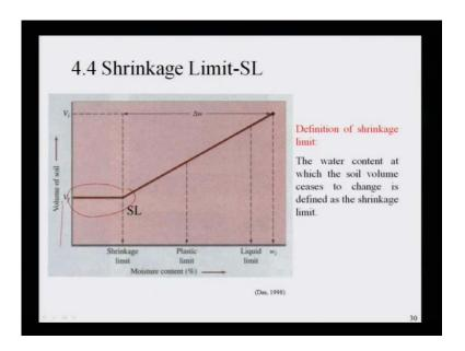
which there is no more change in volume of soil .So, basically if this is my shrinkage limit beyond which there is no more change in volume, volume remains constant. So, this shrinkage limit will give this state that means solid state of soil and
