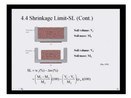
we have discussed about the shrinkage limit. How to find it out? We can find it out by taking the volume of soil and water and making it dry and find it out mass and volume of soil, dry soil from there you can find it out shrinkage limit.
