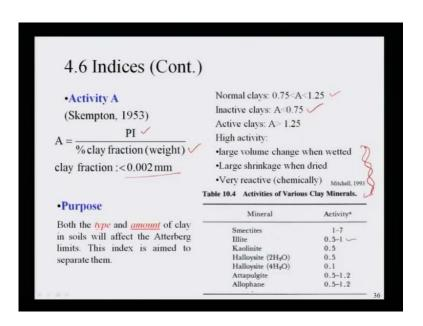
Now, next indices is your activity is like a it it has been given by Skempton 1953 it is called A, activity means A it is your plasticity index P I divided by percentage of clay fraction by weight. So, clay fraction has been taken as far this Skempton generally, if it is soil particles passing through the shape 0.022 mm that means 2 micron shape below this if soil fraction, soil particles passing this is called clay fraction.
