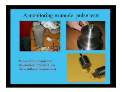
Now, if you look at here this is basically I am showing a bender element, how it has been placed inside this triaxial cell equipment. So, there are two methods one is your in suit methods by seismic downhole or by means of seismic crosshole, you can find it out shearwave velocity if you do not have any shear wave velocity data, in field you can conduct also in the laboratory either in undisturbed sample or in remolded sample.
