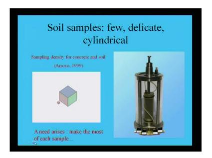
in laboratory particularly this use of bender element in laboratory also by using bender element you can measure dynamic property of soil by means of means you can measure this shear wave velocity in a triaxial cell. You can place your bender element and go for test you can find it out. What is the shear wave velocity of the soil? Now, make
