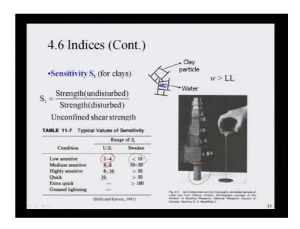
Then next index indices is your sensitivity S t this sensitivity is specially use for clays. So, sensitivity S t is strength undisturbed that means strength in undisturbed divided by strength in disturbed conditions so, if you look at here undisturbed a is your undisturbed
