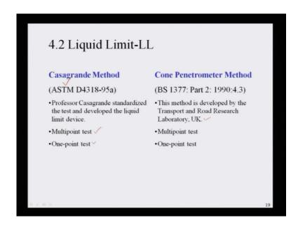
Then it has been measured by means of two standards, one is your American Society of Testing Material (ASTM), American Society of Testing Material that is D4318-95a. Another is your Cone Penetration Method - that is BS1377: Part 2: 1990:4.3. So it is basically Casagrande method, comes from Professor Casagrande standardized this test and developed this liquid limit device and we can find it out there are multi point state test or one point test.
