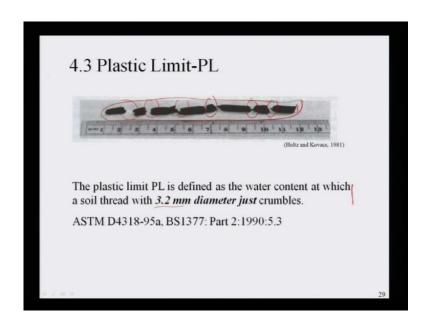
In the next part, is your in atterbergs limit, that is your plastic limit. The plastic limit is define as the water content at which a soil thread with 3.2 mm diameter just crumble. What does it mean? That means similarly, you take 100 to 200 gram of soil mix with water like 5 percent or 10 percent or may be 15 percent water with mixing this water.
