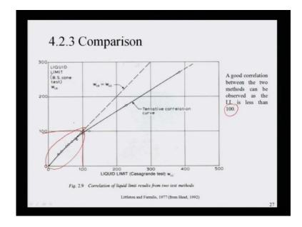
So, these are all if you look at liquid limit by BS cone method. By BS cone method and tentative correlation curve provided by this Clayton and Juke, 1978. If you look at here, means a good correlation between two methods can be observed as the liquid limit is less than 100. A good correlation between this, correlation and your liquid limit by means of British Standard cone test, it will be achieved.
