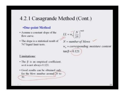
Yes, there are methods that means, this is called One-point method that means assume a constant slope of the flow curve. That means liquid limit is equal to w n N by 25 tan beta, N is equal to number of blows, w n is equal to corresponding moisture content, tan beta has been taken as 0.121. That means, this slope it has been derived from this statistical results of 767 liquid limit tests.
