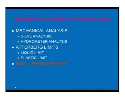
Test on CNS material cohesive non swelling soils, CNS is cohesive non swelling soils it is required these are the following tests. It means some mechanical analysis in the mechanical analysis its sieve analysis and hydrometer analysis. Then ATTERBERG limits, liquid limit and plastic limit and swell pressure test. (Refer Slide Time: 01:14)
