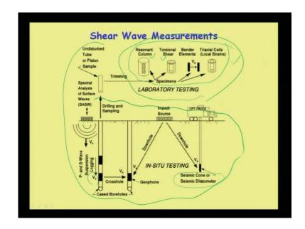
This part we cover in-situ, next class onwards I will start what are the different laboratory testing to get dynamic properties of soil reasonant column, torsional shear bender element and triaxial cell. This I will start from next class.
