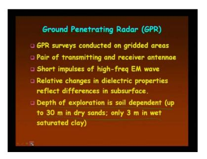
Now, ground penetration radar GPR on particularly, it has been conducted on gridded
