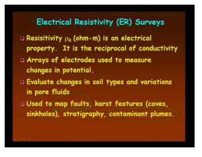
Resistivity unit is as I said earlier ohm meter is an electrical property. It is the reciprocal of conductivity, arrays of electrodes used to measure changes in potentials, evaluate changes in soil type and variation of pore fluids used to map fault, look at here what purpose it has to be used. It is used to map fault, any fault is there below ground you can find it out, caves, sinkholes stratification, contaminant plumes.
