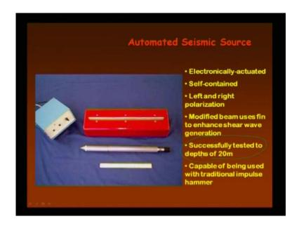
Now, there are different automated seismic source electronically actuated or self contained, left and right polarization, modified beam use fin, successful tested depth up to 20 meter, capable of being used with traditional impulse hammer. These are all seismic piezocone has been made it automatic seismic automated seismic source that can be automated instead of hammering you can start this automated source also.
