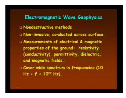
Electromagnetic wave geophysics, non-destructive methods, non-invasive or conducted cross across surface, measurement of electrical and magnetic properties of ground, electrical means with respect to resistivity or with respect to dielectric or magnetic field.
