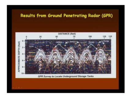
These are all examples of ground penetration radar. Typical results from ground penetrating radar GPR system, approximate versus distance these are pipes, tanks you can easily locate it where it is there exactly at what depth.
