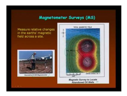
Electromagnetic magnetometer with this magnetometer earth magnetic field across a site you can change the magnetic field below the ground surface based on that, this is basically used to find it out is there any oil, is there any natural source, natural resources below the ground surface.
