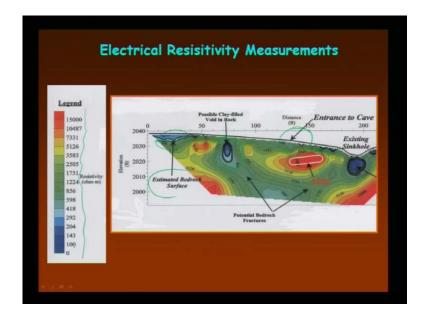
This is one of the typical result I am showing this from electrical resistivity. Where is the cave? This is the entrance of cave, where it is located exactly you can find it out. Is there any sinkholes below the ground? Yes, there is sinkholes. Where it exactly the sinkhole is existing. Then, is there any possible voids in soil or rock? Yes, we are getting possible voids and is there any bed rock where exactly bed rock? This is the surface where the bedrock is there.
