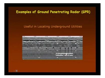
Locating underground utilities, is there any drainage pipe below the underground that you can easily locate it.
