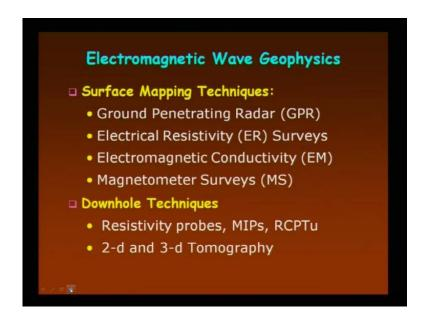
For surface mapping technique most advanced one is your ground penetration radar GPR then, second one is your electrical resistivity, third one is your electromagnetic conductivity, fourth one is your magnetometer surveys and downhole techniques resistivity probe or MIP s 2 d and 3 d tomography.
