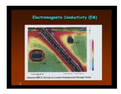
Then electromagnetic conductivity EM by means of varying magnetic field also you can classify. This is latest one this pipe, tank or anything you can find it out.
