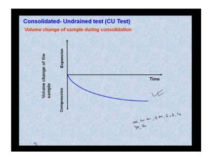
Now, how this volume change will look? You can measure volume change sample during the consolidation, that means, during consolidation compression, with this compression with time means, with time you can, 1 minute, 2 minute, 4 minute, 6, 8, 16, 30, 1 hour, these are all equal, means double the time interval you can measure this. How much is your compressor and volume change of the sample, you can plot it, that this is called your compress, means consolidation graph.
