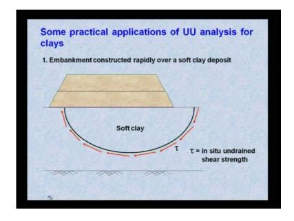
Now, you come back to some practical applications of UU analysis. That means, in field conditions what are the conditions where you will prefer for this test, unconsolidated-undrained test, first is your case one.
