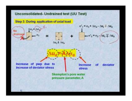
Now, stage 3 or step 3, during application of axial load what will happen? There is no drainage, so sigma 3 plus sigma delta sigma d. Delta sigma d is nothing, but your sigma 1. If I write in terms of change in pore water pressure, so it will be delta sigma 1 sigma 3 plus delta sigma d minus delta U c plus minus U d U c plus minus U d.
