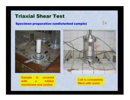
Once again I am repeating this, once you place this sample in the base and place inside the cell, this is your triaxial cell, place inside the cell, that means, this confinement means, confinement, you apply confining pressure by means of water filling inside. (Refer Slide Time: 34:00)
