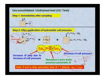
Unconsolidated-undrained UU test - step one, immediately after sampling means, before placing in the triaxial immediately after the sampling has been done, that means, it lost, it lost your confining, that means, sigma c is equal to 0, so there is no overburden or no confining pressure, so this is 0.
