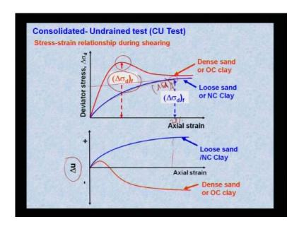
Now, stress-strain relationship during shearing, so deviatoric stress delta sigma d, it will increase with (()), means stress will increase with axial strain. So, you will get at the peak, you will get deviatoric stress at failure f and similarly, axial strain also change in pore water pressure, with respect to volume change versus axial strain. This is nothing, but your volume change versus axial strain and this will be your for dense sand or over consolidated clay.
