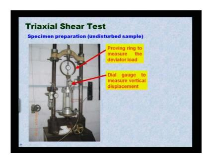
If I go my earlier of this triaxial test equipments, look at here, this confinement comes from here in the cell. In the cell, the confinement sigma 3.
