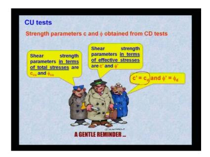
CU tests strength parameters, c and phi obtained from CD tests. Shear strength parameters, in terms of total stresses, it is said C cu and phi cu. Now, shear strength parameter, in terms of effective stress, it is effective means prime, once prime is their C prime or phi prime, it means, it, it denotes to effective stress.
