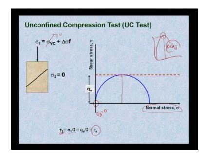
What you are supposed to get? You will get if, if I go for unconfined compression test, you will get, this is your normal stress del sigma. If I come back here, look at here, sigma 3 is equal to 0. That means, there is no confinement; that means, sigma 3 is equal to 0. If I want to plot this Mohr circle, that means, sigma 3 is equal to 0, means it will start at origin. In this case, it will be sigma 3 is equal to 0; that means, if I draw the Mohr circle, this is my sigma 3 and sigma 1.
