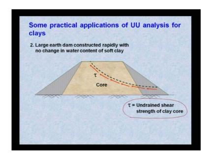
Now, example two, large earth dam constructed rapidly with no change in water content of soft clay. There is no change in water content in the soft clay means, in that soft clay this water content will be remain same. In that case, you will be getting undrained shear strength of clay. That means, in this case, you will go for UU test in the laboratory.
