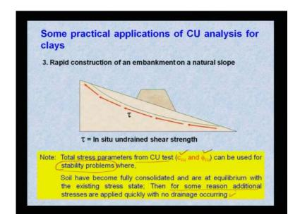
Third example, rapid construction of an embankment on a natural slope, this is an embankment, the construction will be rapid, that means, this construction is not slow enough, so that development of pore water pressure or change in volume due to water, it will, it will occur. So, because of rapid, this generation of our development of pore water pressure will not occur. So, this will be example, 3rd example, for practical application of CU analysis.
