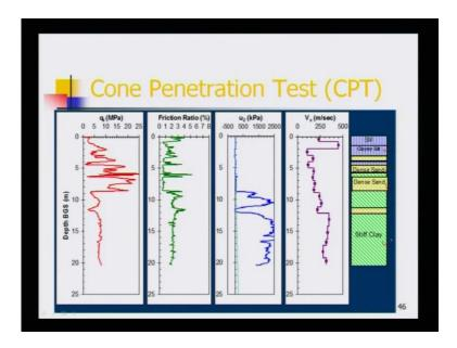
Now cone penetration resistance with these, it is shown again in terms of Mega Pascal, all these and velocity depending upon that. The classification has been made with this cone resistance, this will be clay silt, and this will be dense sand, dense sand and stiff clay.
