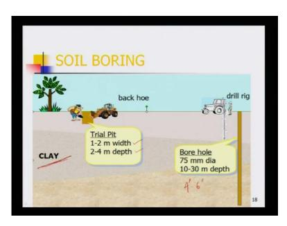
Another part I have already explained this soil boring, but I want to show this figure wise means, open pit or trench you can do it trail pit, up to you can limit is up to one point generally 1 point 1 to 2 meter width and 2 to 4 meter depth. It can be done kind of a clay, where you can very easily collect a soil sample by means of a trial pit. Bore hole, as I
