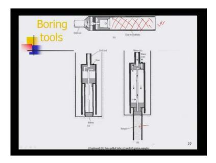
Another boring tool is thin wall tube; if you look at their thin wall tube, this is generally used; this is in India generally used. Once you in the drill rod, once you attach this thin
