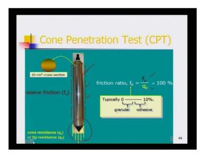
Now, this cone penetration test; I explained also in blackboard also. If you look at the figure, this is 10 centimeters cross section of cone, and this will be measured by means of sleeve friction; these are all sleeve friction, and cone resistance or tip resistance, you can measure it here. So, friction ratio f R is equal to f s by q c into 100 percent. Typically it will be 0 to 10 percent of this, has been used.
