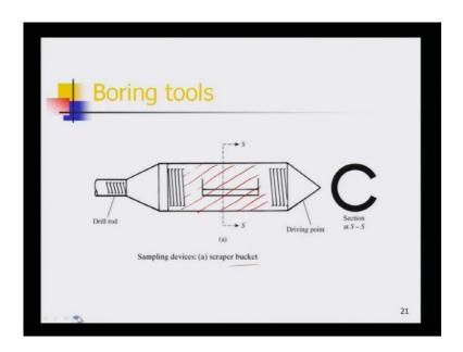
You see, these are all your sampling tools, boring tools, sampling tools, there are different kinds of boring tools, that is your scraper bucket and driving, this is your driving point. Once you push it inside, it will collect the samples in inside, I will show lateral in detail, the dimension required for different kinds of soils; what kind of soil, this is required.
