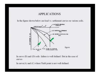
If you look the load versus settlement diagram or this, if this kind of curves are there, where you can get failure load easily.
