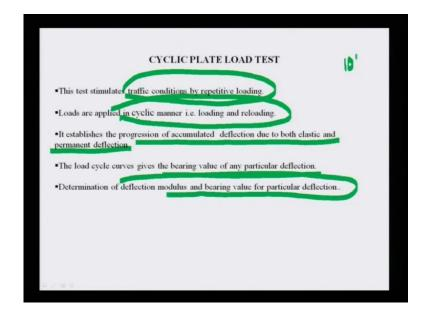
Then, next question is, with this plate load test, will it be possible to conduct a cyclic plate load test? Yes. Generally, cyclic plate load test is required to simulate traffic condition by repetitive loading. Load are applied in cyclic manner, loading and reloading. That means, first set of load whatever you applied in plate load test.
