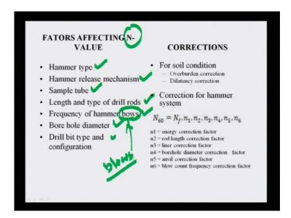
What are the factors affecting N-value in field. What type of hammer used, it depends upon the hammer type. Also, how the hammer release, it is manually or may be mechanically operated. What is the sample tube used, length and type of drill rods, frequency of hammer bows. Then, bore hole diameter, drill pit type and configurations. Then, frequency of hammer blows. Sorry, this is wrong, this will be blows.
