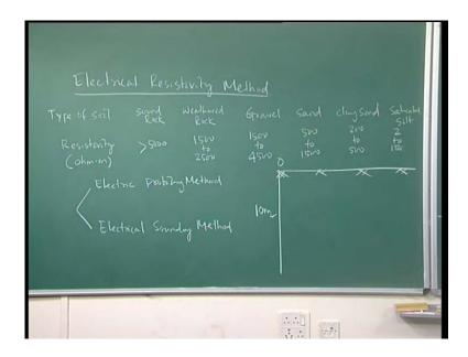
Suppose, this is the range, where the depth of exploration has to taken up to ten meter from the ground surface, zero to ten meter depth of exploration has to be carried out. Suppose, in zero meter to ten meter, you are going to carrying out, sub soil exploration.
