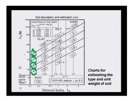
Now, that is another, it is plotted with dilatometer index E D versus the material index I D, task for estimating type and weight of soil. If you see this, there are range A, B, C and D types of soils. From this range, you can find it out, if you know E D and material index you can find it out, what kind of soil, where is the range, you can easily find it out.
