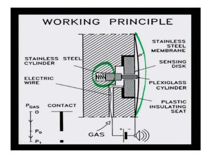
It is connected by means of a stainless steel member, inside there is a spring and plexiglass cylinder also there, and plastic insulating seeds are also there. By means of gas, ones it enters. So, it will try to expand outside. The moment it expand outside, so soil will give resistance. So, this resistance or the sigma three, you can get it, how much this spring. Spring will be compressed, from there we can get it.
