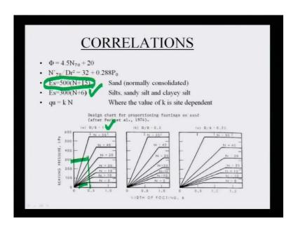
Then correlations, it has been also explained also earlier. For sand, normally consolidated sand, you can find it out E s soil, five hundred into N plus fifteen. For sand silty, silt and clay, you can find it out, E s equal to three hundred in to N plus six.
