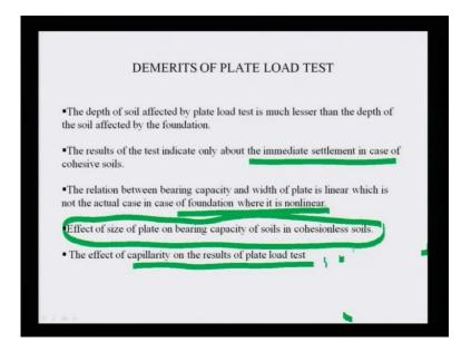
What are the limitations, this part I am not discussed. What are the limitations in plate load test, the limitation is depth of soil affected by plate load, much lesser than depth of soil affected by foundation. If I say, this is my plate. So, depth only affected by very small area, and this is my footing. That means, it is affected by much larger area.
