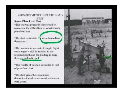
That is, another test it is called screw plate load test. This test was primarily developed to overcome the difficulties, associated with this plate load test. The test is suitable for loose to medium dense sand. The instrument consist of single flight earth auger which is inserted to the required depth, and the loading is done through hydraulic jack, you can see it here.
