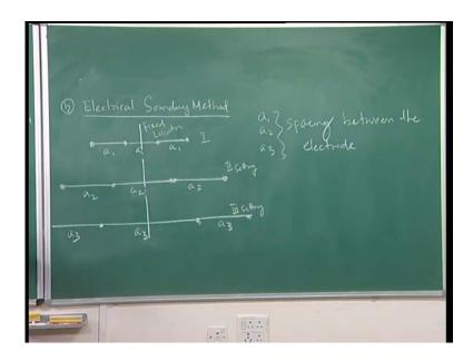
These are a one, a two, or a three. These all are spacing of electrodes. Spacing between the electrodes, you can vary the spacing between the electrodes. So that, you can reach, up to the depth of exploration.
