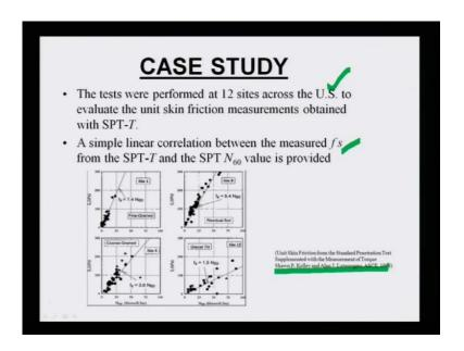
So, basically it has been, there are case studies means, test were performed at twelve sites across in U.S. united states to evaluate the skin friction measurement obtained, with S P T and T. Based on that skin friction measurement, a simple linear correlation between the measured skin friction and the S P T-T is provided. So, this has been given by shawn A T L nineteen ninety eight, they propose correlation between the measured f s from S P T-T and S P T N.
