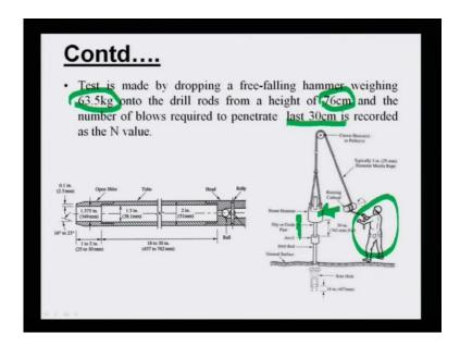
You can see this schematic diagram of the standard penetration test, if you look at here. Now, this is your hammer, then it drops height of seventy five. This is sixty five in indian condition, it is used as per a h t mit is sixty three point five, and height of fall is seventy six, but some other standard it is, sometimes seventy five, sometimes it is sixty five also.
