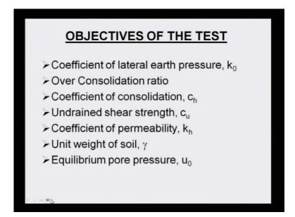
Now, what you are suppose to get from this test. Coefficient of lateral earth pressure, this coefficient of insitu conditions. I mean in insitu condition coefficient of lateral earth pressure k zero. Then over consolidation ratio, coefficient of consolidation c h, undrained
