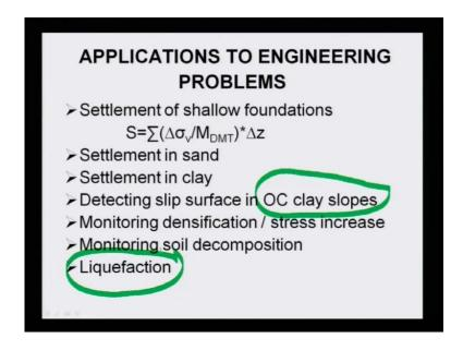
Application to engineering problem, settlement of shallow foundation, you can also get settlement in sand, settlement in clay, then detecting slip surface in slopes, and also as well as, as you are measuring pore water pressure. You can also determine liquefaction as well.
