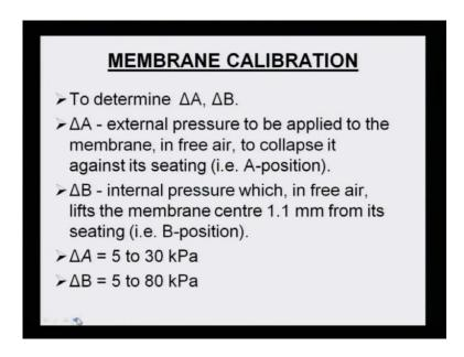
And there are two parameters required to find it out. One is your, how much external pressure applied to the membrane. Then is your internal pressure, which in free air lifts
