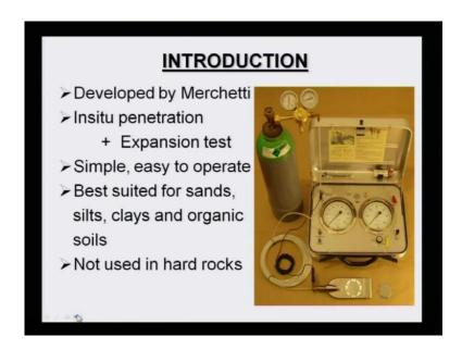
Next is your dilatometer test, means dilatometer test has been developed by merchetti. It is basically insitu penetration as well as expansion test, it is simple and easy to operate. So, best suited for sands silt clay and organics soils, it has not been used for hard rock.
