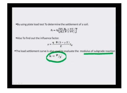
Now, as I said, using plate load test, you can find it out, settlement of soil, or also you can get influence factor. Another one is your, load settlement curve used to evaluate modulus of sub grade reaction means, k value you can find it out, p by y. From this, you can find it out, modulus of sub grade reaction.
