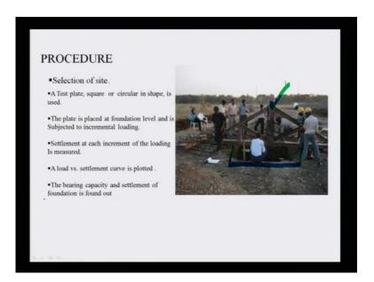
Now, look at this figure, in real field, there is loading platform, a pit has been made from here to here, pit has been made, and this is the loading platform, and this plate load test has been carried out the photograph, I put it directly.
