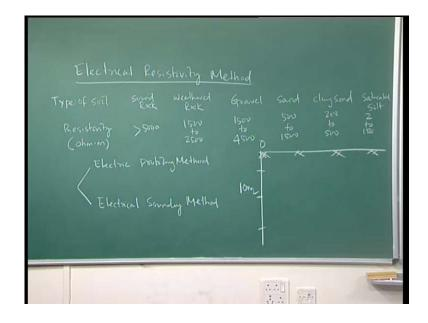
Let us say, every two meter interval. For two meter interval, then you said, from the fixed location. So, a one should be two meter. Then similarly, next four meter, a two should be four meter. Because in electrical resistivity, the resistance you can measure up to a distance, that is equal to spacing between these electrodes. So, a one is two meter.
