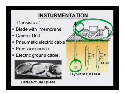
And if you look at this part, you can say, if you look at here, the layout of this D M T, it consists of a blade, this part is your blade. Now come back to this instrumentation, it consists of blade with a member, this is the blade, generally with a member. Then control
