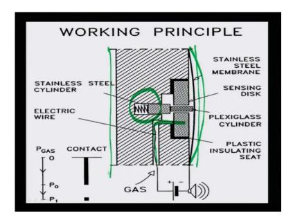
The moment by means of gas, it will try to expand. Ones it expand, what will happen, here the soil is there. With this soil resistance, then this spring will be either expand or may be contract. Based on the spring resistance, you can find it out sigma three.
