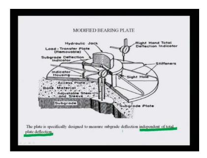
This plate is specifically designed to measure sub grade deflection independent of total plate deflection. Look the difference, it is specially designed to measure the sub grade deflection which is independent of total plate deflection.
