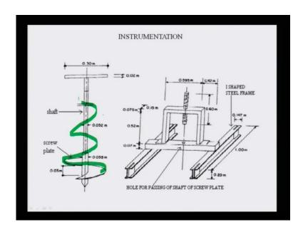
Look at here, screw plate, a plate it is screwed, it is put in a shaft, so it has been posed. Then the plate load test has been done, by means of the procedure, earlier procedure for regular plate load test, same procedure has been applied. Here the settlement observed is more accurate.
