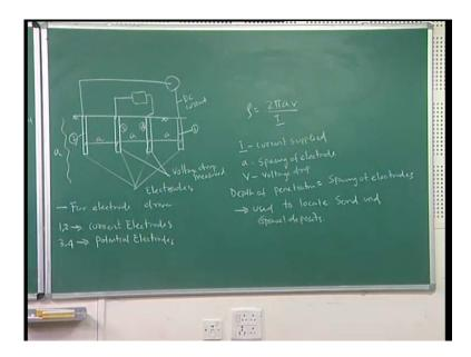
Now, in case of electrical profiling method, what happen, if this is the ground surface (( no audio 03:18 to 03:34)). Now, these are current electrodes, these are your electrodes and this is equal distance say a a and a.
