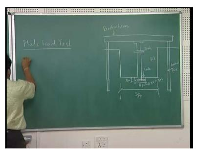
Next part is your plate load test. (No audio from 00:20 to 01:39) Plate load test has been conducted to find it out the bearing capacity of plate, as well as settlement profile of this plate, from these plate load test results, this can be co-relate to or maybe you may find the plate load test means bearing capacity of footing, and as well as settlement of footing.
