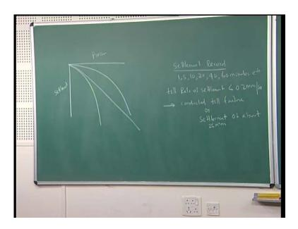
So, settlement record settlement record is 1 minute, 5 minute, 10 minute, 20 minute, 40 minute, 60 minutes, and rate of settlement till rate of settlement less than 0.2 mm per hour. How far this test can be conducted - it can be conducted till failure or settlement of about 25 mm. What is the output pressure, here it is settlement.
