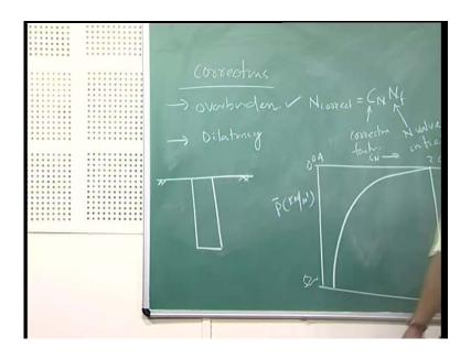
Now, there are two corrections: One is your overburden, other is your dilatancy. Why these corrections required? If you look at this from SPT - standard penetration test, how the standard penetration test has been conducted. First, up to that depth bore hole has been made.
