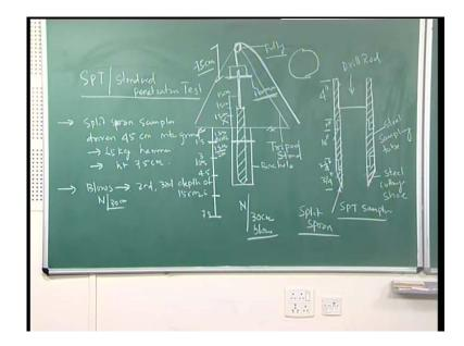
Now we will start, first one is standard penetration test - first one is SPT or it is standard penetration test. How it looks? (No audio from 07:15 to 08:15) Now, this is your it goes to drill rod - 4 inch, 1 inch, 18 inch, 2 and 1 4 th inch, then 3 by 4 th inch. This is your steel cutting shoe, this is steel sampling tube, so this is called SPT sampler. Now, how it looks SPT sampler.
