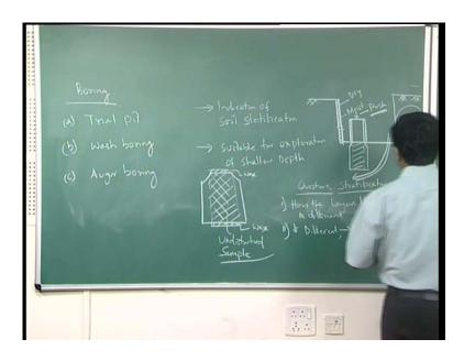
Once you make it out, the casing pipe (No audio from 21:03 to 21:11) it collects undisturbed sample, by means of wax by means of wax both the ends by means of wax, you make it water tight, this is your wax water tight, so that moisture content preserved - moisture content preserved. Then this undisturbed soil sample can be taken to the lab for soil testing, this about this sampling tube samples, this we will discuss after this part of the boring, then come back to next is your wash boring.
