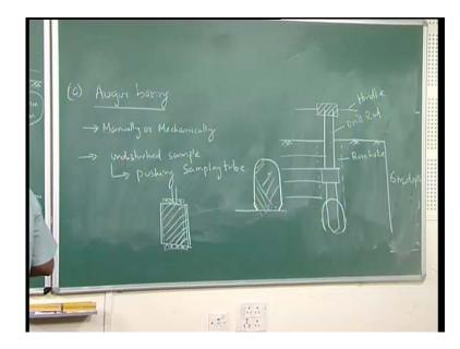
Manually or mechanically operated, undisturbed samples obtain pushing pushing sampling tube. Now, if you look at this auger boring if you look at this auger boring, generally this may be this may be manually or mechanically done, this is a drill rod shaft, it is connected by means of auger.
