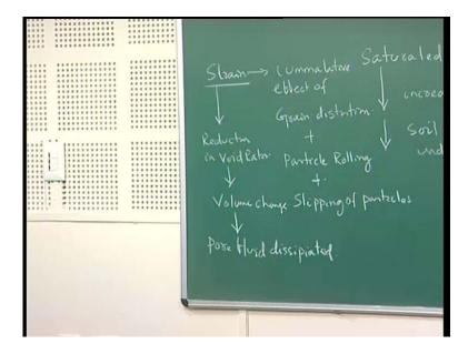
So then from here because of this, there will be reduction in void ratio or we call volume change or pore fluid dissipiated. Now with this let us start with this consolidation and consolidation settlement.
