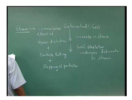
Now let us say saturated soil; it is acted by increase in stress. So then, then soil skeleton undergoes deformation or it is called strain. Now, come back to strain. It is cumulative effect of one is grain distortion then, plus particle rolling then plus, slipping slipping of particles.
