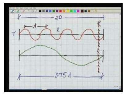
Now, in order to do that, we will go to this diagram. Again, in this case, this is the distance 2D (Refer Slide Time 41:28), a wave, as seen here by the red colour, is fired from our transmitter. It goes to the reflector somewhere here (Refer Slide Time 41:44), and then finally to the receiver- let us say the receiver is here (Refer Slide Time 41:58). I
