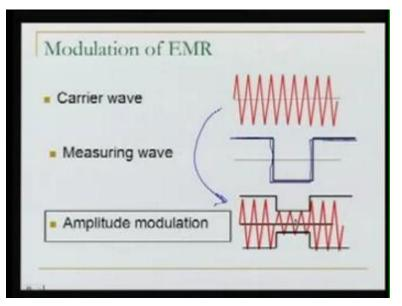
The very first modulation is 'amplitude modulation'. In the case of the measuring wave, as you can see here, this is the wave (Refer Slide Time 09:19), so it has its signal like this (Refer Slide Time 09:21), so we modulate the carrier wave in such a way that the carrier wave carries the signal of the measuring wave, as you can see here in a very rough diagram (Refer Slide Time 09:27). So here, the carrier wave has been modulated.
