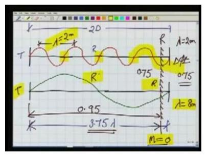
Now here, in the figure also, here in this figure, I had increased - we started with a lambda of 2 metre; as you can see here, we started with a lambda of 2 metre. Then, I took a lambda which was 4 times that one, and this lambda, if it occupies, in one full wavelength, the entire distance starting from transmitter to the reflector and again back to the receiver, if this entire distance is covered in less than one full wavelength of this lambda, then, in that case, our M has to be 0.
