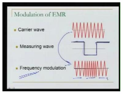
Similarly, there could be another modulation - this modulation is the amplitude modulation, the another one could be 'frequency modulation'. What we are doing? The signal which you want to send as the measuring wave (Refer Slide Time 09:51) is being sent by modulating our carrier wave in frequency. As you can see, the frequency is changing here (Refer Slide Time 09:59), and this change in the frequency is carrying the signal of the measuring wave.
