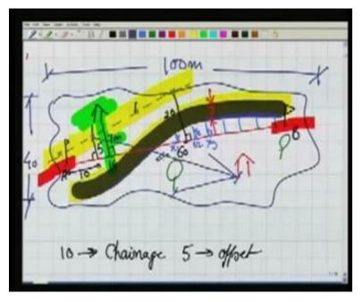
For example, there in the ground I take some observations which are independent of the survey, which we are not using in the survey, which you are not using in the plotting. For example what I can do, I can also measure the distance between this tree and the building here. I can measure the distance between the telephone pole and a building here. Well these two distances are measured independently there on the ground.
