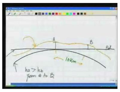
I will give one more example - here is the earth (Refer Slide Time 11:31), as you can see – that is the surface of the earth, and this surface here (Refer Slide Time 11:39) is the geoid, and here is the flat plane which is tangential to the geoid at this place. Now, in this example, what we are seeing: if we plot our point, let us say, or rather, we measure the height of the point - that is, the point A (Refer Slide Time 11:59) and a
