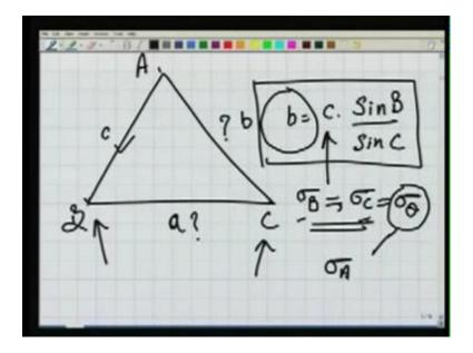
Well, we have a triangle and this triangle is A, B and C, where length c is known. It is known because this is the length which is either coming from the previous computations or is the base length which is being measured here. So, we know this length. Now, the job is to determine length b and length c, sorry length a. What these are? We want to compute these. So, for length b, we have seen previously also and we can write it as c sin of B and sin of C.
