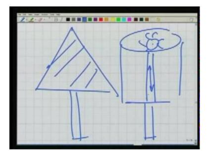
Similarly, we can have a thicker ranging rod. I can say you know a cylinder, a wooden cylinder and it is painted white and black or red and white, and we are using that as a signal something to bisect or we may have the signals which are of you know a kind of cone. Then, we have the stand of that. We can use it for the signal because we can see it from a distance very far. We can have instead of cone, a cylinder, a big cylinder and again we can see it from a distance.
