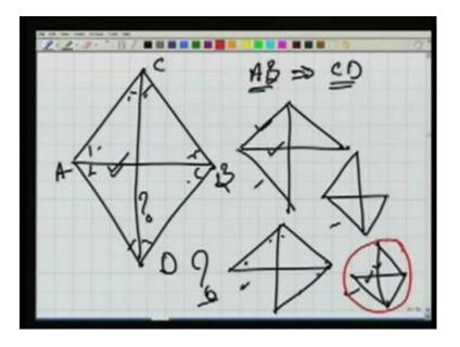
There is one more concept, which we can answer by the strength of figure and that is if we have let us say a triangulation figure like this, and in this A B is known while C D is unknown and this is known, all these angles are measured. As in the case of the triangles, it is starting from AB. You want to compute CD. Now, it is only one triangulation figure, one triangulation network is not like here.
