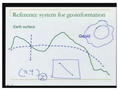
Because of the non-uniform distribution of mass, the - if I draw it again - because of this non-uniform distribution of the mass, for earth, the geoid will be of a shape which will be different. Now this shape of geoid is not mathematically defined, so even if we project our point onto the geoid, we do not know anything between what is happening there. In case of our simple map, each and every point is defined. You take any two
