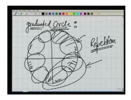
Now, the next error that we are going to is error due to graduated circle. Now, in the previous case I was giving you example of the horizontal plate, but the same is true for the vertical also. If there is eccentricity in vertical circle and the vernier, again we need to take the observations for vernier A and vernier B. In vertical we were saying vernier C and vernier D take their mean the error due to eccentricity will be eliminated.
