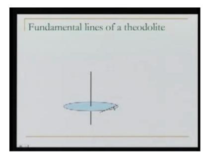
Then this redline here is the axis of the bubble tube. We have a bubble tube and for this bubble tube we can define the axis, which is tangent at this middle point this is the axis of the bubble tube. Then further, because we have not only the horizontal circle, but on top of that the vernier frame with these two index, because we are making use of these index a and index b or we can say vernier a and vernier b to take the readings.
