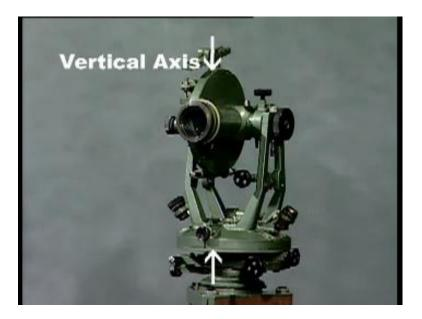
Vertical axis means, if I show you here in the theodolite I am rotating this theodolite, it rotates about a line here that is the vertical axis, then we have the horizontal circle. So, this circle is the horizontal circle, where we have the graduated circle, where we read the angle values.
