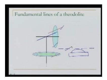
So, there is another axis which we can define, this is the axis of the vernier frame or we say inner axis. So, this dotted line here is the inner axis. If you go further or we have the horizontal axis, this is the horizontal axis about which we can rotate the telescope. Well, we go further this is the line of sight. Line of sight means, the line which is here in the telescope.
