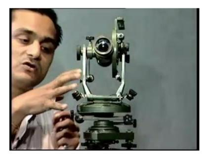
One more error, for example, let the sun is on this side here. So, only part of the instrument is being heated. Now, if only part of the instrument is being heated, what will be the reason? What will, what might happen? The graduated circle may expand in one part while it is not so in the other place. So, again that might lead to some error.
