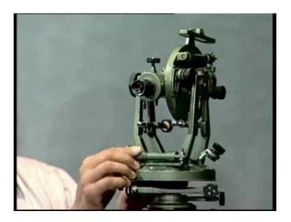
How do we ensure it? We will make use of the altitude bubble. We have seen on the index frame, there is an altitude bubble. This altitude bubble is more sensitive, more sensitive than the plate bubble. So, after centering this plate bubble, again using the foot screws we centered this altitude bubble.
