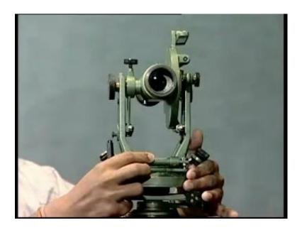
So, far we have seen the methods for measuring angles in horizontal. Now, we will see the method for measuring vertical angle. Now, what is the meaning of vertical angle? The meaning of vertical angle is, for any object we are measuring the angle of this, from the point of observer with the reference as the horizontal line. So, that is the horizontal plane. So, from this horizontal plane we are measuring this angle to an object there. So, that is my vertical angle. We have seen this definition.
