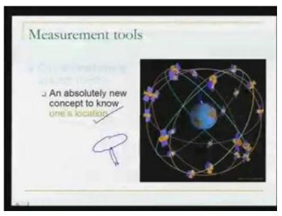
What the GPS is: in the case of the GPS, as you can see here, all around our earth we have around 24 - I am saying 24 at the moment though it is not exactly 24, it is more than that - number of GPS satellites and these satellites are orbiting the earth in such a way that at any moment of time, if you are standing anywhere, you can see at least 4
