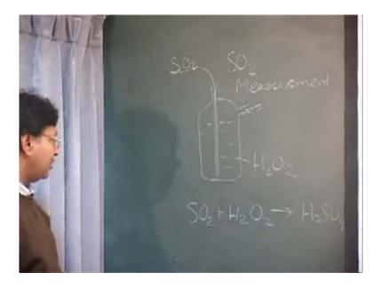
When you want to measure  $SO_2$  from the stack or in the atmosphere, you take  $H_2O_2$ , this may be outlet. Put  $SO_2$  in there; this  $SO_2$  will quickly make  $H_2SO_4$ . Is it balanced? It should
