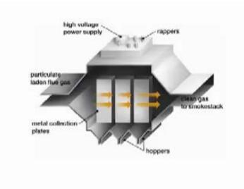
But before we go into that, I was just showing you if these are the plates, they are parallel plates, there are many plates and in between the plates, there is something and that will be used for charging the particles.
