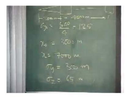
This is your Taj Mahal somewhere here. This distance is 300 meters and what is this distance from center to this? 4 kilometers. 4 kilometers, so 4,000 meters. So your x is equal to really 4,000 plus 3,000 or 7,000 meters. The sigma<sub>y</sub> spread by the time it goes to Taj Mahal will be equal to... I have to find out at 7 kilometers. All agreed? This is your 2, 3, 4, 5, 6, 7, 300; sigma<sub>z</sub> starts from 5, 6, 7, F, go back. How much?
