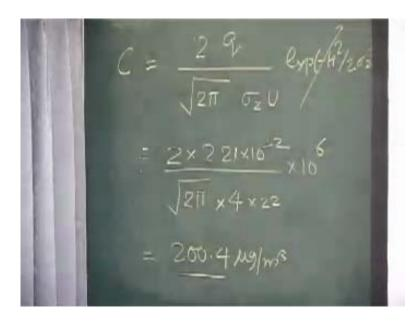
This will be my... 2 times what is the q? 2.21 into 10 to the power...? —2. 10 to the power —2. U we will take the same as 4 meters per second and we must find out sigma<sub>z</sub>. How far is it from the...? 1 kilometer. Distance is... take this... 22 or so. This is in grams but I want in micrograms.
