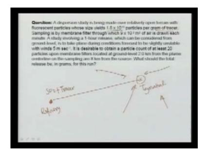
I will not call this example difficult, but it will require some understanding of the problem. The problem reads like this: a dispersion study is being made over a relatively open terrain with fluorescent particles. We are trying to do some measurement of the fluorescent particles whose size yields 1.8 into 10 to the power of 10 particles per gram of tracer. Let me also give a little background of tracer studies and what tracer studies are.
