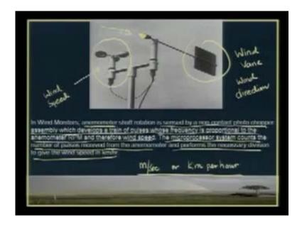
Now, we are talking about measurements. What you see on your screen is a photograph of a wind measurement system. This side I will circle (Refer Slide Time: 25:16) and that is called wind anemometer and this measures the wind speed; this one is called wind vane and what it measures is the wind direction. Although we do not ourselves manufacture these – experts do it, we should at least know the underlying principles as to how the wind speed is measured.
