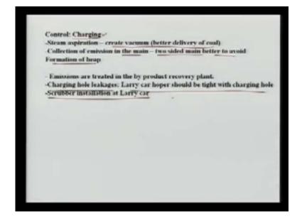
Sometimes on the top of the larry cart, a scrubber is provided. The emissions that are taking place are passed through the scrubber process. After charging, the hole must be luted – luted means closed seal. You all know M seal. This is called luted and luted means you put some chemical around this – mostly, it is clay that is used so that the charging hole become airtight.
