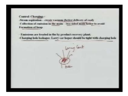
Emission is treated in the by–product recovery plant and once the emissions are collected from the main, they go to the treatment plant. Some people also talk about leakages: the larry car hopper should be tight with charging holes. As the larry car is charging and there is a hole here, this must be made be tight; otherwise, what will happen is that there will be leakages from here. This is the larry cart, for example, and this is the oven. This fitting should be very tight.
