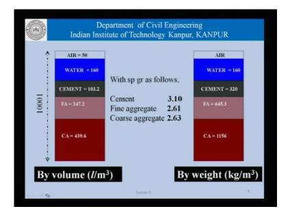
Now, when we went through that example we found this to be the volumetric distribution of the different materials- air, water, cement, fine aggregate, coarse aggregate, all these volumes been given in liters per cubic meter. We also had with us this weight distribution of the materials in terms of water, cement, fine aggregate, and coarse aggregate.
