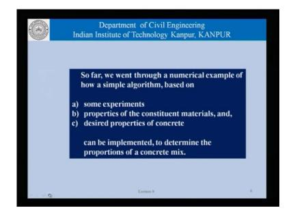
Now, the limitations or the assumptions in our example, where that we were working with the very simple concrete mix, that is only having the basic ingredients- the fine aggregate that is sand, coarse aggregate- cement and water. Of course, we assume that we will have a certain amount of air. So, the example that we used can be used for air entrained concrete as well as non air entrained concrete depending on what kind of air entraining at mixture we use or we do not use.
