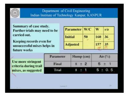
The way to do that is this. If we go to this example what we have done is, with this water cement ratio this is what we had initially, this is what we had finally, and we hope that we got the right results. What we need to do, to ensure that the mix is robust and is able
