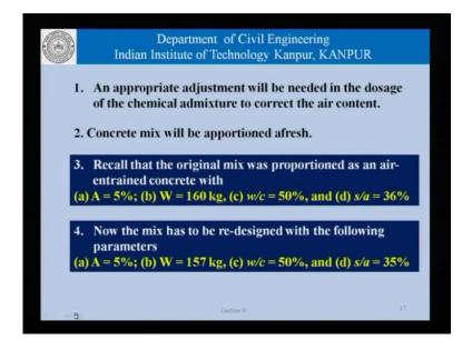
Now, to recall what we have done, an appropriate adjustment will be needed in the dosage of the chemical admixture to correct the air content. The concrete will be apportioned afresh. And beginning with this example that we had, we will now work with the parameters- air content is 5 percent, water content is 157, water cement ratio is 50 percent, and s by a is 35.
