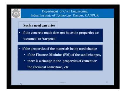
And, that need can arise if the concrete made does not have the properties we assumed or targeted. Or, it can arise if the properties of the materials being used change. That is, for example, the fineness modulus of the sand changes. A concrete project does not get completed in a day.
