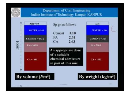
And, if you proportion the mix, this is what happens. We have air, we have water is a 144, we have cement which has been reduced, we have the coarse aggregate is still being kept at 400, we reproportion this concrete mix with 144 kgs of water, and this what we get, by volume and by weight.
